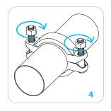
**NOTICE:** Uneven tightening may cause gasket to pinch. Gasket should not be visible between segments after bolts are tightened.
