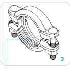
Apply thin coat of lubricant Keep foreign particles from adhering.
